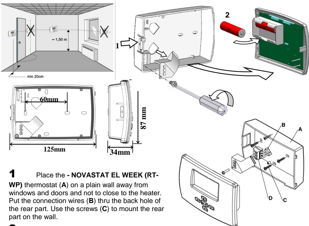
**1** Place the - NOVASTAT EL WEEK (RT-WP) thermostat (**A**) on a plain wall away from windows and doors and not to close to the heater. Put the connection wires (**B**) thru the back hole of the rear part. Use the screws (**C**) to mount the rear part on the wall.
